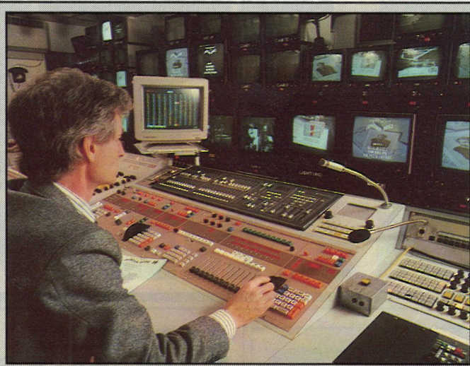
London's Greenwood theatre, the television studio that is home to Channel 4's Tonight with Jonathan Ross , has a twin lighting installation. It was planned to install a Strand Galaxy 3 lighting control system, but the production company, Channel X, felt it might not be sufficient for live rock acts. The solution was to mount Strand's latest MX24 board next to the Galaxy 3. MX24 can introduce chases and flash channels individually, as well as acting as a back-up to the Galaxy if necessary.
